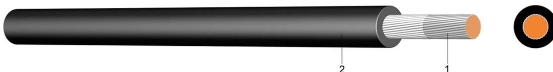
**Construction:** 1 ..... fine-stranded tinned or bare copper
