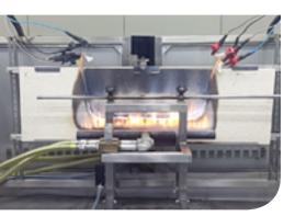
EN 50200 Annex E Test for resistance to fire of unprotected small cables for use in emergency circuits (Optional Water Spray Protocol)
